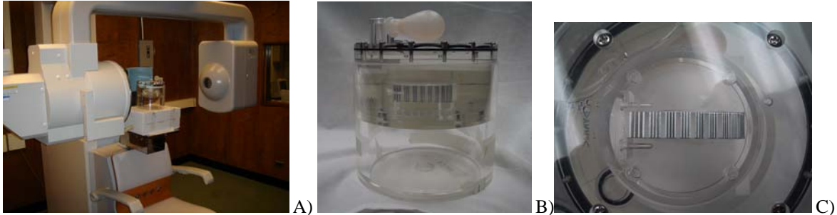
Figure 02 – A) C-Phantom in position to be scanned by the CBCT, B) full view of the C-Phantom, and C) close up view from the top showing the 9 series of metal lines used to assess image resolution.
