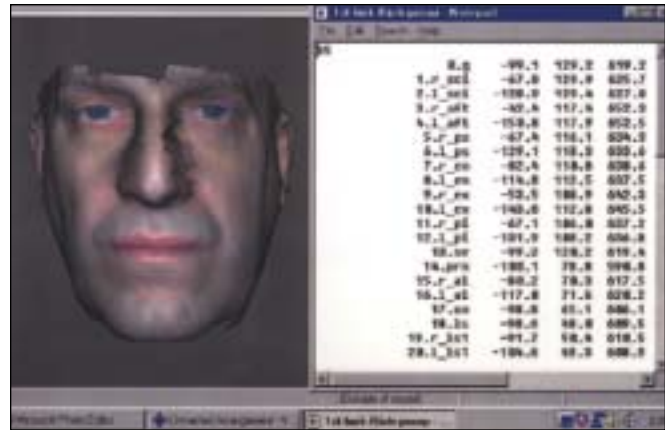
Fig 3 The 3D coordinates (landmark name and x, y, z columns from left to right in table, right) of the soft tissue landmarks were collected by direct digitization of stereophotogrammetric images (see Table 2).
